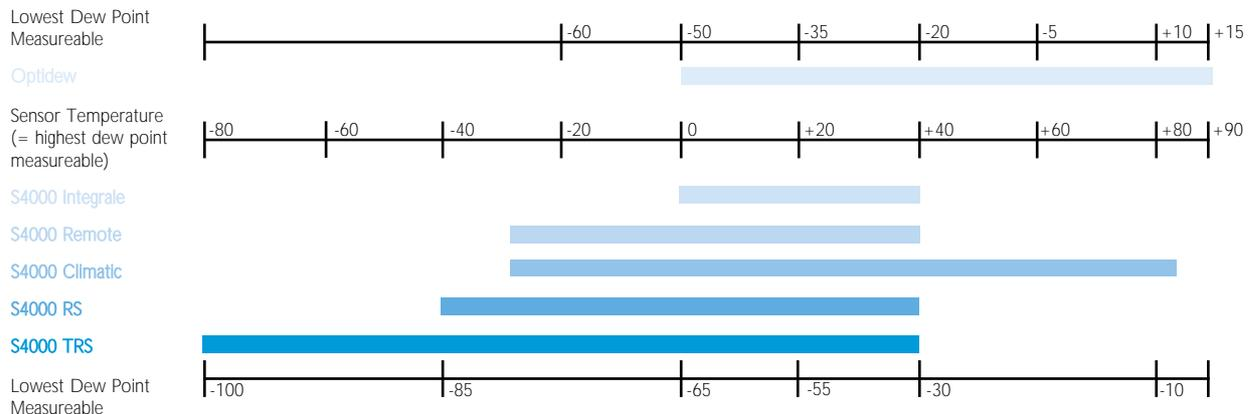
**Note:** for Optidew Climatic Sensor the lowest dew point measurable = 10 °C less than the standard sensor (shown above).
