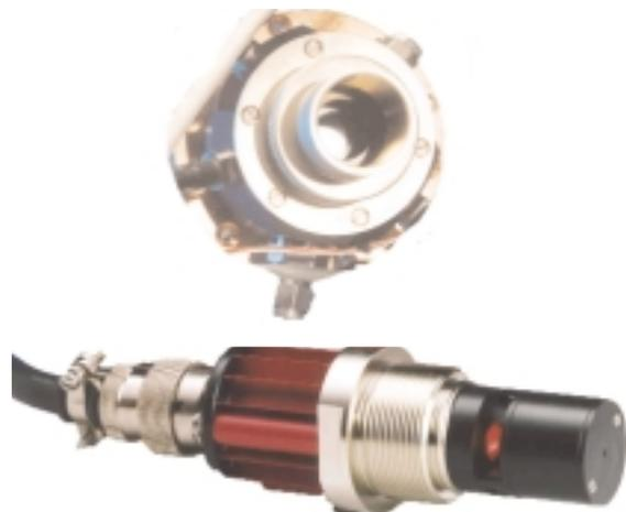
of light reflected from the mirror surface is used as a feed input into the instrument control electronics to modulate the cooling power applied to the Peltier. The mirror surface is then controlled in an equilibrium state whereby evaporation and condensation are occurring at the same rate. In this condition the temperature of the mirror (measured by a platinum resistance thermometer) is equal to the dew-point temperature of the gas. This process is shown diagrammatically in Figure 1.
