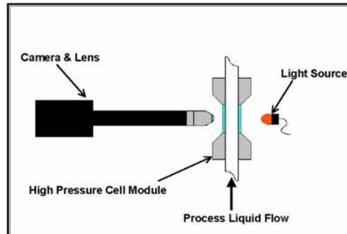
ViPA operates by freezing a single frame of the video image and analysing the objects present. A database of information is built by rapidly acquiring and analysing sequences of these frozen images.
