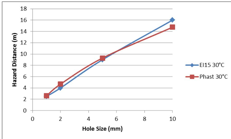
Figure 1 - Comparison of EI15 versus Phast for 30°C ambient temperature cases
