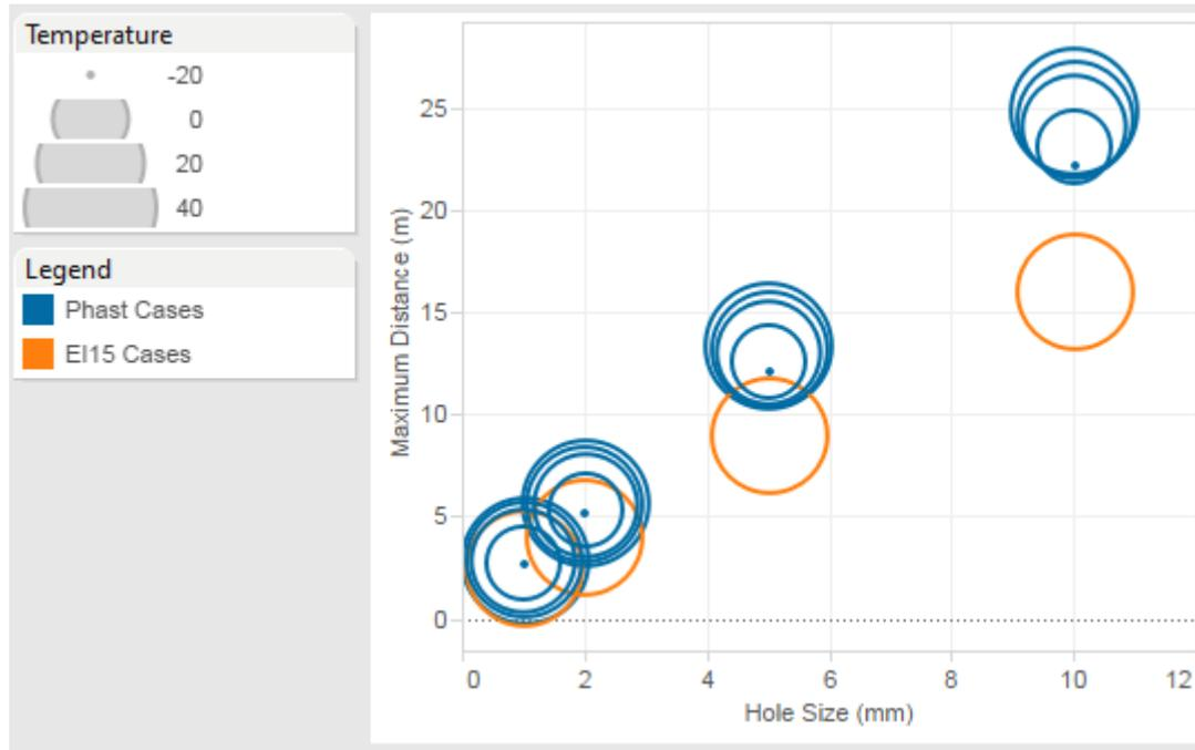
Figure 2 - Hole Size, Hazard Distance and Ambient Temperature 3-D scatter plot
