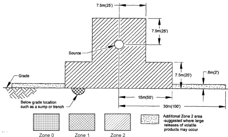
**Figure 2 – Generalised Method Solution for Heavier than Air Gas or Vapour from Secondary Sources of Release**
