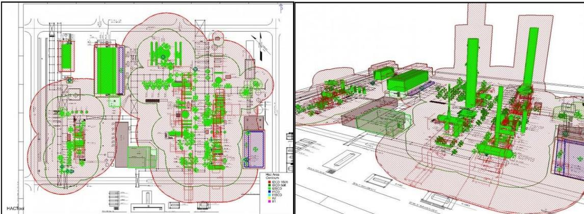
**Figure 3 – Plant Classification using the Generalised Method**
