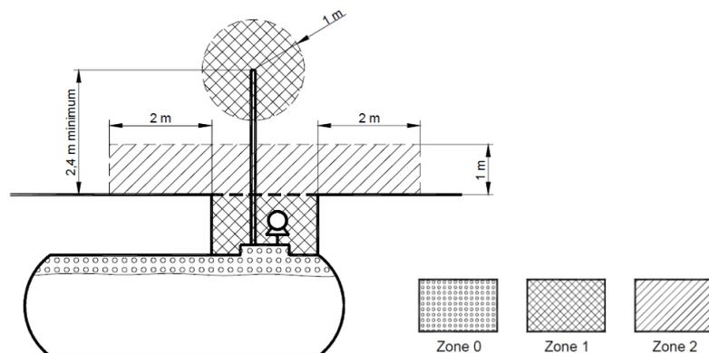
Figure 1 – Typical Classification of an Oil/Water Separator
