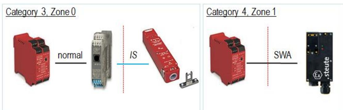
As with the E-stop example, two techniques are shown here – one using an intrinsically safe approach to provide for zone 0 requirements, and one using an Ex-de rated solenoid to provide for Category 4 requirements.
