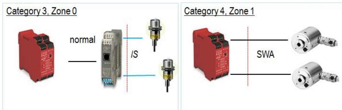
As with the solenoid interlock and E-stop example, two methods are shown here, using different protection techniques. Note that Category 3 is applicable to both – this is a function of relay operation; Category 4 is not commonly used in connection with speed monitoring.
