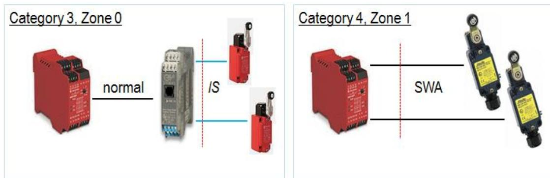
As with E-stops, we are dealing with simple devices connected to the Galvanic Isolator shown in the Category 3, Zone 0 approach on the left. This means that while the limit switch still needs to be safety rated, it does not need to be Ex-i rated.
