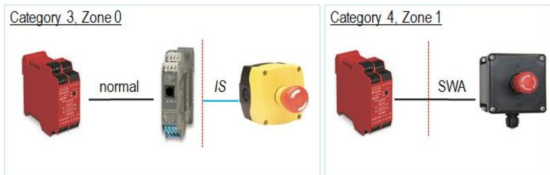
The Category 3, Zone 0 solution shown on the left uses a safety relay and a dual channel galvanic isolator (IS barrier) in the safe area, with intrinsic safe
