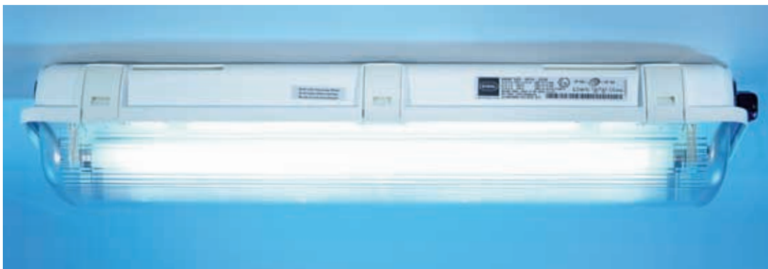
Figure 9: Explosion Protected Luminaire 6600 Series for Use in Zone 21 (Category 2D) and Zone 22 (Category 3D).
