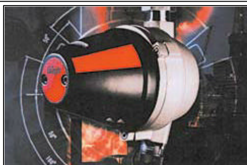
Figure 2 and Photo 2. In an IR gas sensor, one IR light beam is of a wavelength that excites a particular type of gas molecule and thus loses part of its energy to the resultant molecular vibrations. The intensity of that beam is compared to a second beam of the original energy, and the differential is used to measure the gas concentration. The Polytron IR is an explosionproof detector for combustible gases and vapors.
