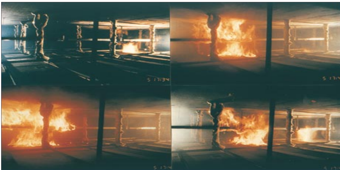
Figure 25 - Flame Propagation, Dripping Fire Balls, and Pool Fires.
