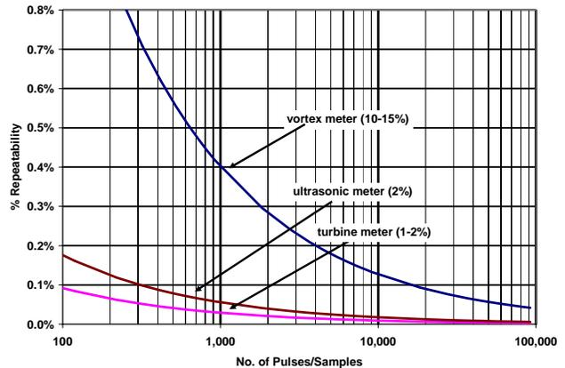
**Figure 3: Predicted Repeatability vs. Number of Pulses/Samples for Varying Standard Deviations**
