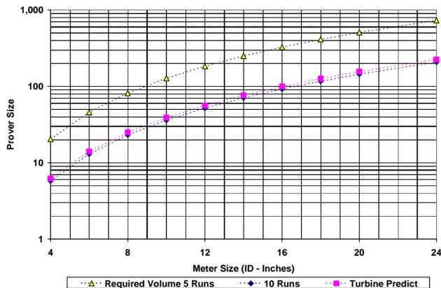
**Figure 7: Prover Volume - 5 Run and 10 Run API Required Repeatability**
