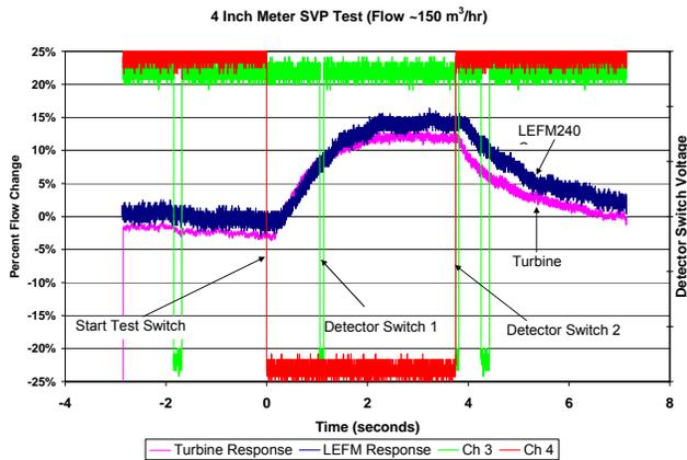
**Figure 9: Flow Rate Changes During Proving-Velocity 20fps**
