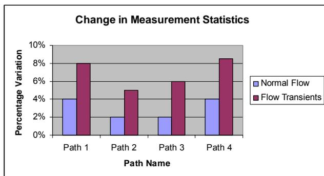
**Figure 10: Meter Reported Flow Statistics during Proves with Unbalanced SVP**
