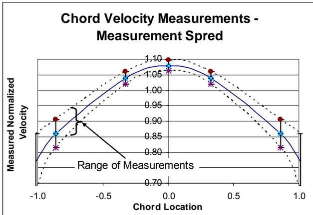
**Figure 2: Velocity Variability vs. Chord Position**
