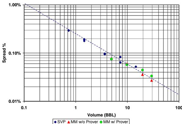
**Figure 4: Repeatability vs. Proving Volume – 4 Inch Meter**
