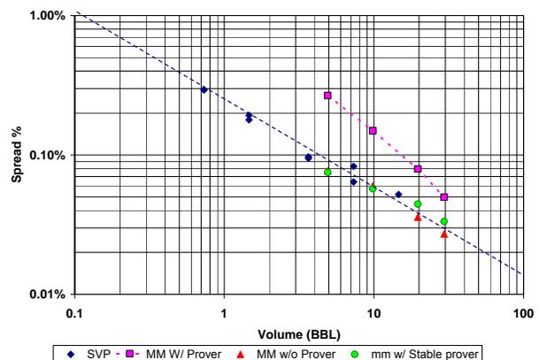
**Figure 8: Flow Instability and Repeatability vs. Proving Volume – 4 Inch Meter**
