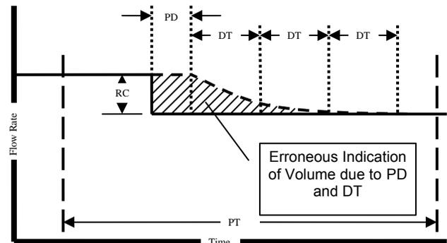
**Figure 11: Potential Measurement Errors Due to Time Response of Meters**
