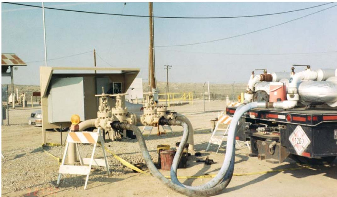
**Figure 5: Compact Prover Test Configuration**
