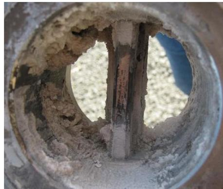
Vortex Meter scaling at the [Talinga Gas Processing Plant](#), the largest Origin operated coal seam gas (CSG) plant in Australia. Calcium Carbonate is clogging the instrument, setting inside like concrete.
