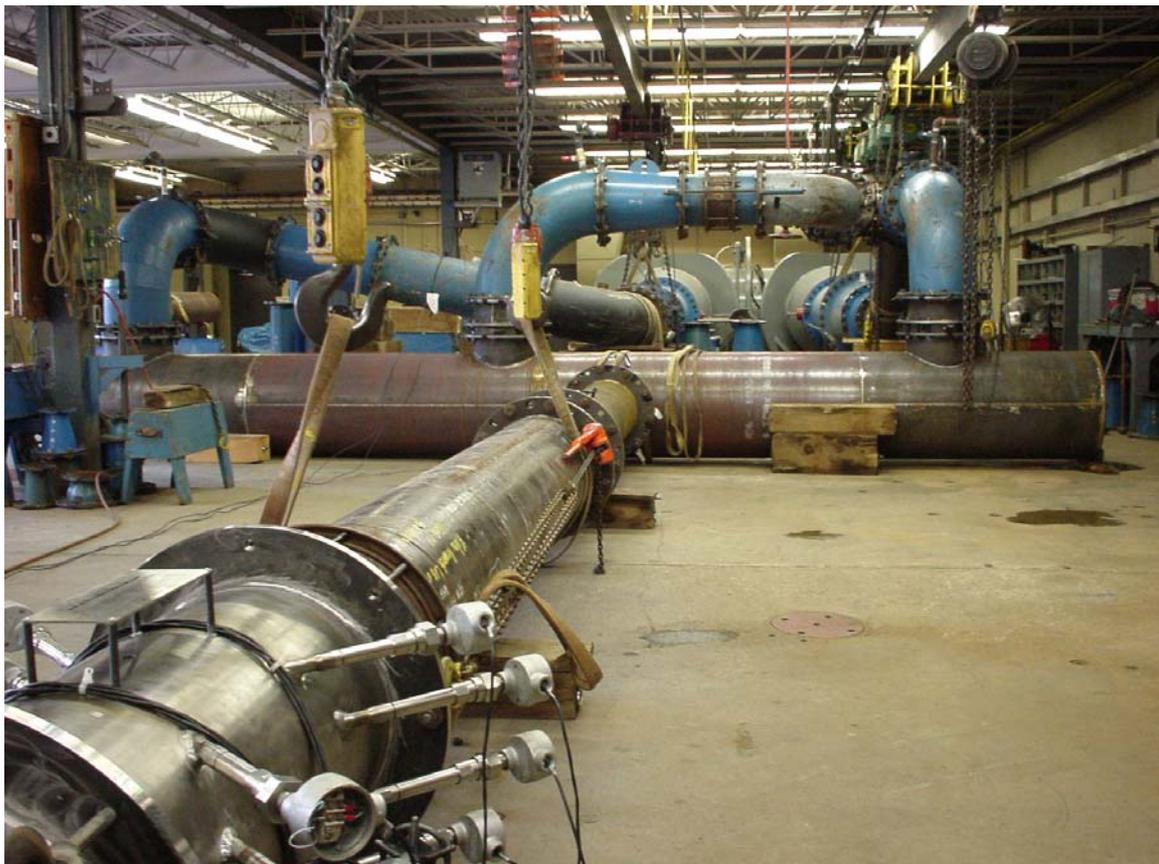
As was noted earlier, the calibration of 4 path chordal meters can be sensitive to transverse fluid velocity, since such velocity components can project onto the chordal paths. Transverse velocity components can change over time if, for example, they are brought about by the distortion produced by a flow regulating valve. Changes in relative roughness can also produce changes in the magnitude of transverse velocity components.
