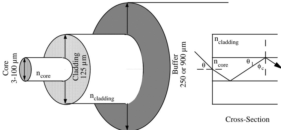
**Figure 1: Cross-section View of a typical Optical Fibre**
