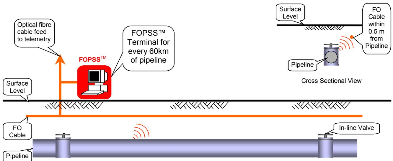
**Figure 3: Fopic™ Pipeline Security System (FOPSS™) – Leak Detection System**
