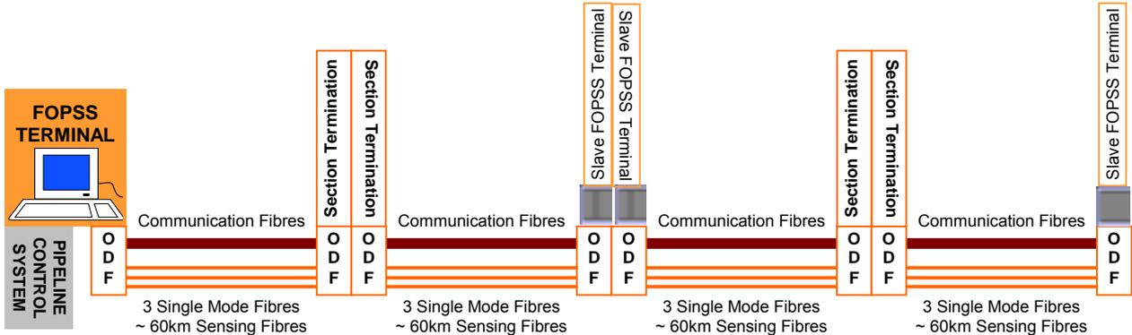
**Figure 4: Multi FOPSS™ Detection System**
