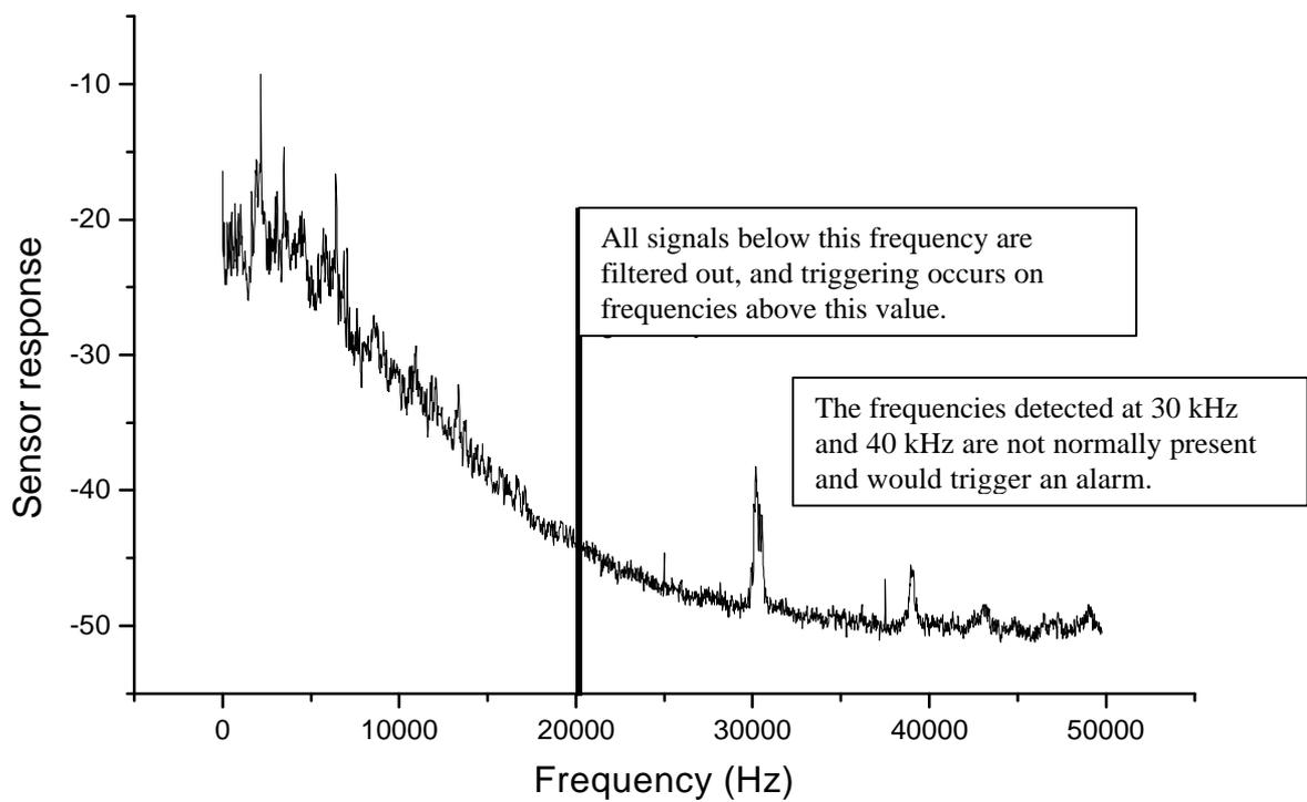
**Figure 5:** Frequency spectrum of actual results of simulated pipeline leaks detected with Foptic™  $\mu$ Strain™ Sensor.
