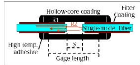
This technology is self-referencing and requires no calibration to measure the absolute gap length (S) in a fibre optic interferometer cavity. If the sensor Gage Length is known, the system automatically provides absolute strain measurements.
