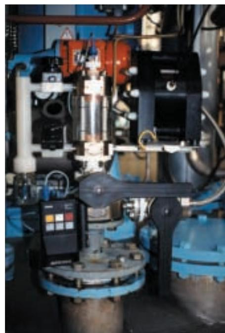
Figure 4: PEV Reactor Sampler.
