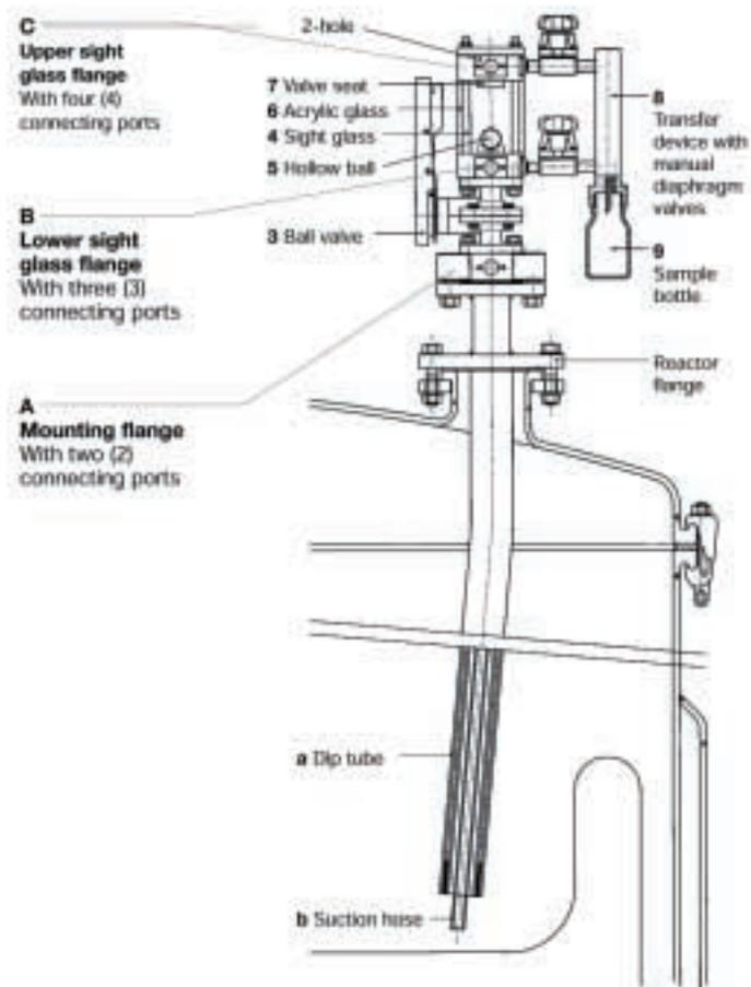
Figure 3: PEV Reactor Sampling.
