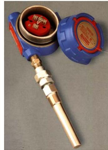
Compared with the low millivolt signals from thermocouples or RTDs the 4 – 20mA signal is robust enough to ignore electrical interference in plant-wide wiring. The signal wire can be copper, not the more expensive, dedicated thermocouple extension wire.
