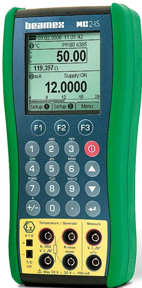
**Beamex® MC2-IS Intrinsically Safe Multifunction Calibrator.**
