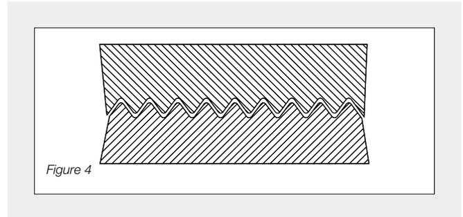
This combination of threads is used extensively in the hydraulics industry and with the correct selection of an appropriate seal material or seal form for the application, high pressures can be maintained.
