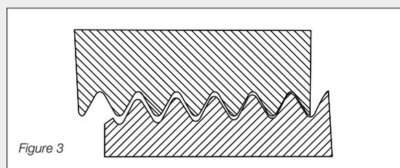
The matching of these threads, with the use of a jointing medium (ie. Teflon thread tape) is sufficient to effect a seal between the mating parts.
