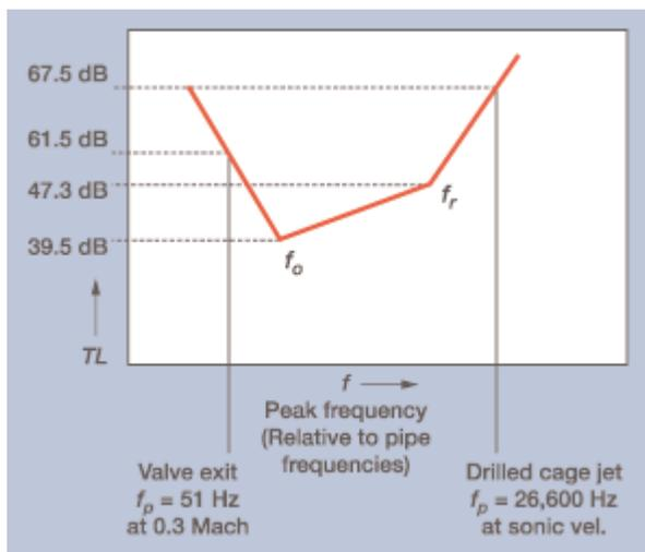
Fig. 3. Due to the relatively large valve exit diameters, expander noise occurs at relatively low frequency.
