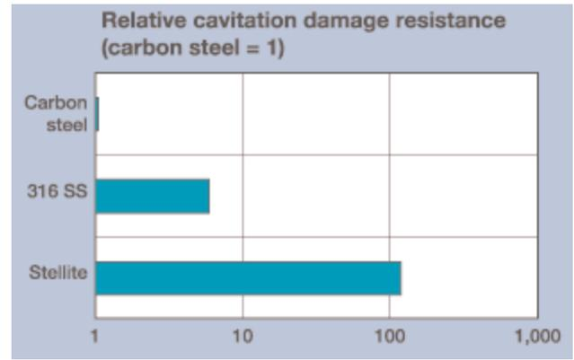
Fig. 7. Stellite is about 150 times more resistant to cavitation damage than carbon steel.
