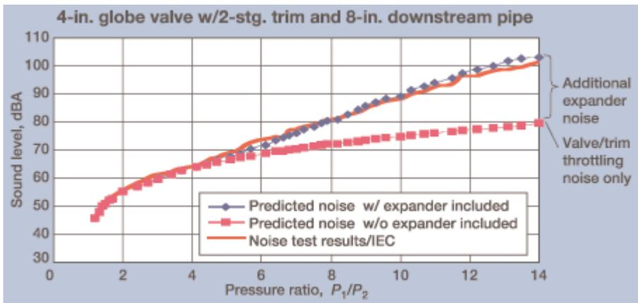
Fig. 1. Calculating expander noise is important, particularly at higher upstream-to-downstream pressure ratios.
