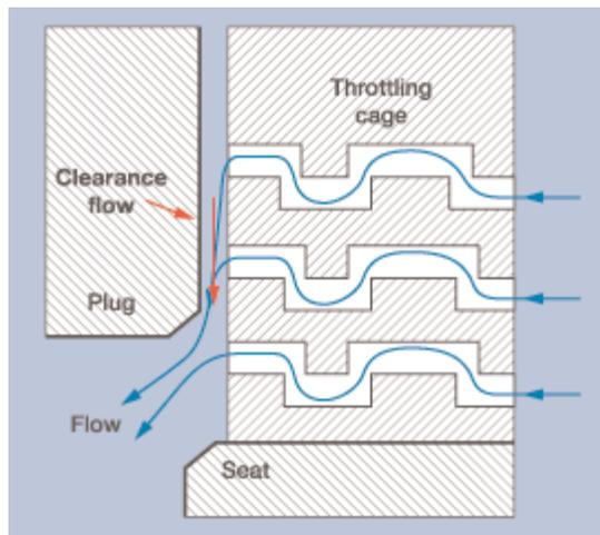
Fig. 4. If clearance between the plug and guiding surface is sufficiently large, the clearance flow path will eventually pose less resistance to flow than the exposed flow paths.
