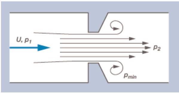
Fig. 6. In control valves, cavitation typically occurs near or at the exit of the valve trim.
