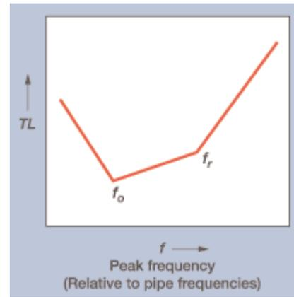
Fig. 2. The scaling relationships for transmission loss reflect the distinct excitation regimes.
