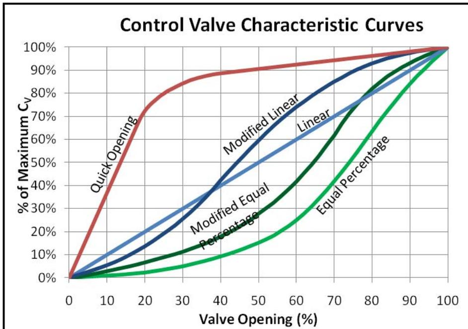
Figure 1: Typical Control Valve Inherent Characteristic Curves
