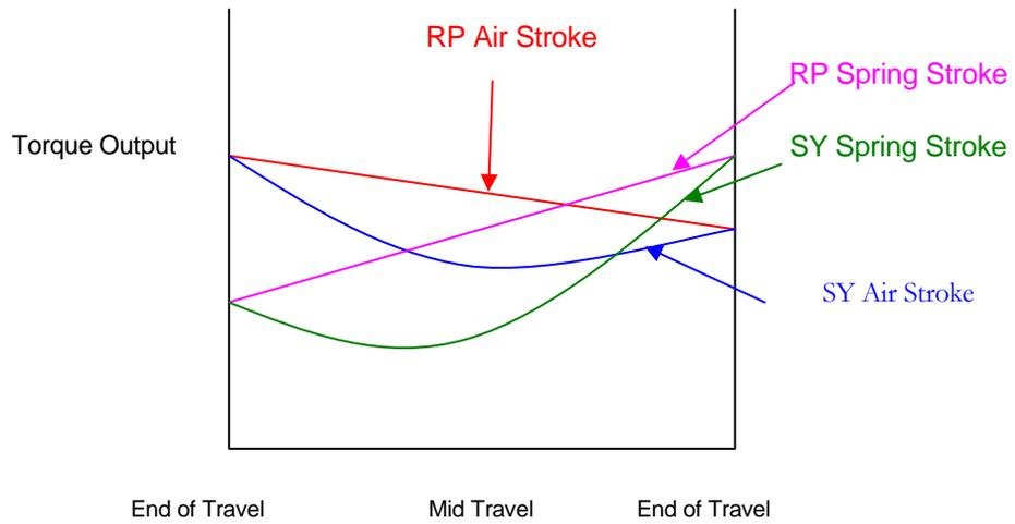
Figure 4: SA actuator torque curve
