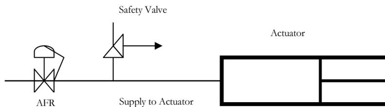
Figure 4: Simplified actuator circuit indicating safety valve
