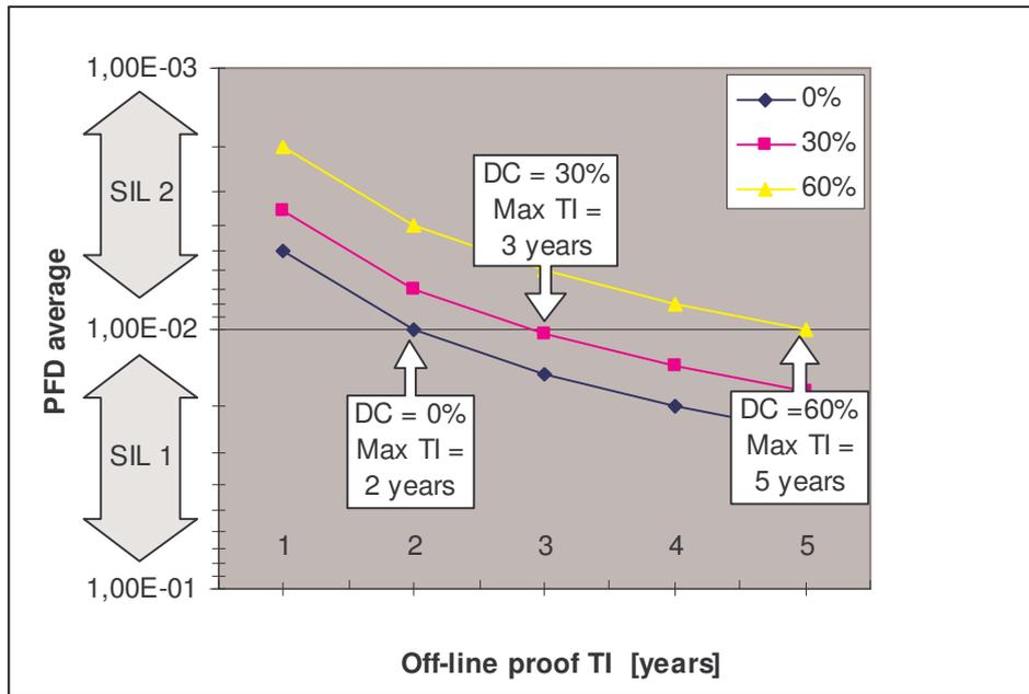
Figure 5 Illustration of the impact of DC on the maximum TI for SIL 2
