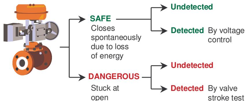
Figure 2 Failure modes of a safety valve
