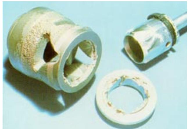
**FIG. 1:** *Improperly specified valves can lead to premature valve failure. Being aware of the many different valve requirements can help you avoid the type of valve damage shown here.*
