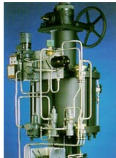
Referencing ISA S75.05 1983 Standard for Control Valve Terminology, these valves should have a linear installed flow characteristic. This means the relationship between the flow rate through the valve, and the travel of the closure member as the closure member is moved from the closed position to rated-travel, will be linear, even though the pressure drop across the valve varies.
